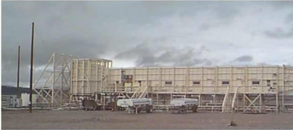
Figure 4. Exterior of Wind Tunnel at the HSC Used for Ammonia Liquid Evaporation Tests
